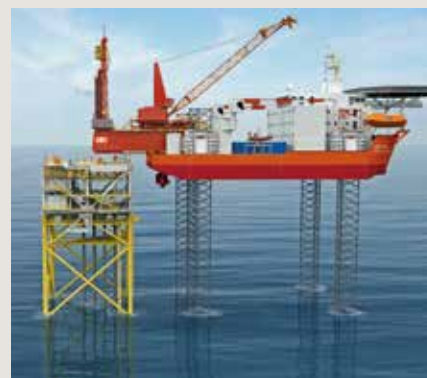
Cantilever workover unit slides from the SESV over the well head.
